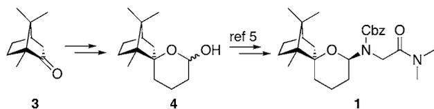
**Figure 2.** Synthesis of camTHP\*-desymmetrized glycinamide **1** from (+)-camphor **3**.
